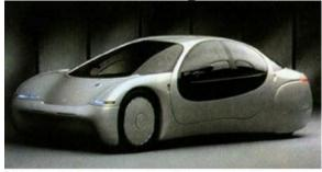
Made entirely from carbon fiber composites, General Motors' Utralite body structure weighs only 420 pounds. The carbon fiber material is half the weight of aluminum -- yet has two times the stiffness. It also has one-quarter the density of steel with slightly better stiffness. However, the material cost alone for the Utralite structure was approximately \$13,000 -- several times the cost of aluminum, steel or fiberglass.
